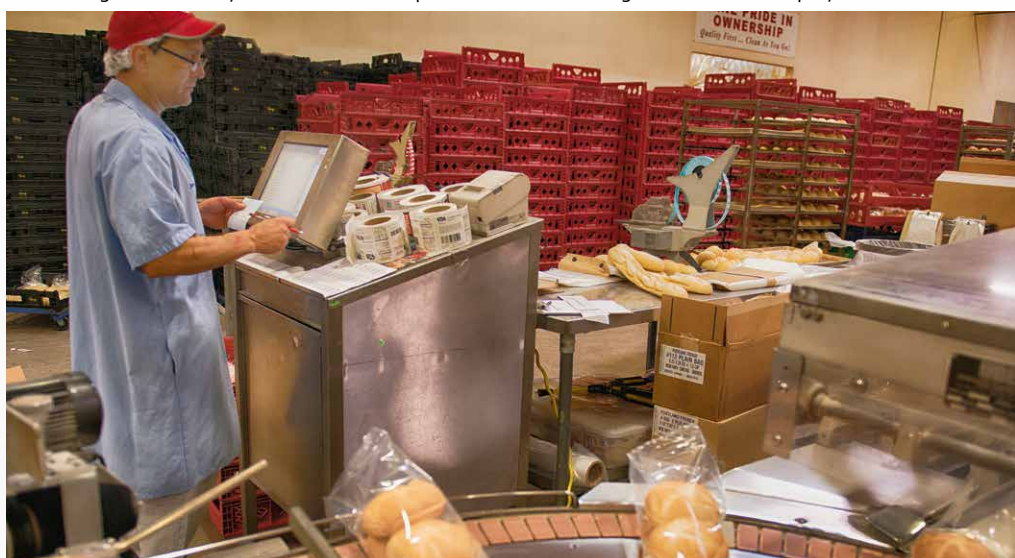
A Portland French Bakery employee uses a noax S15 industrial touchscreen PC to monitor products and print labels in real-time
